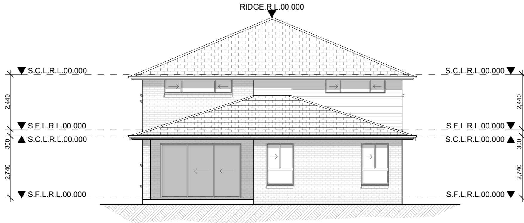
Rear Elevation Elevation 2 scale 1:100
